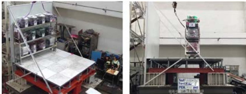
Fig. 6 Wafer/reticle cart implemented on the shake table (Photos courtesy of NYCU)
