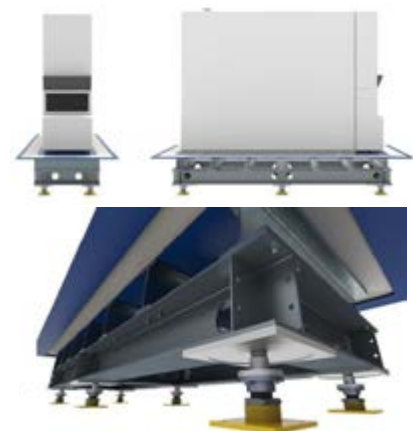
Fig. 3 Illustration of VDF on Isolation Platform w/ Friction Pendulum System (FPS) (photo courtesy of NYCU)
