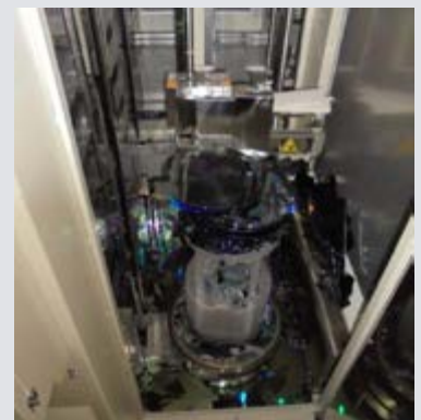
WIP Wafers and quartz tubes breakages inside the Vertical Diffusion Furnace
