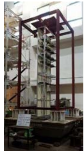
Fig. 4 Stocker and frame implemented on the shake table (Photos courtesy of NYCU)
